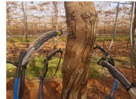
Sapflow monitoring (3 vines/sub-plot, probe depths 10, 15, 20, 25 mm)
