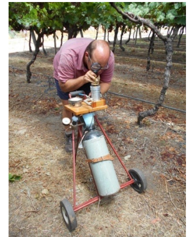
Grapevine water status (pressure chamber)
